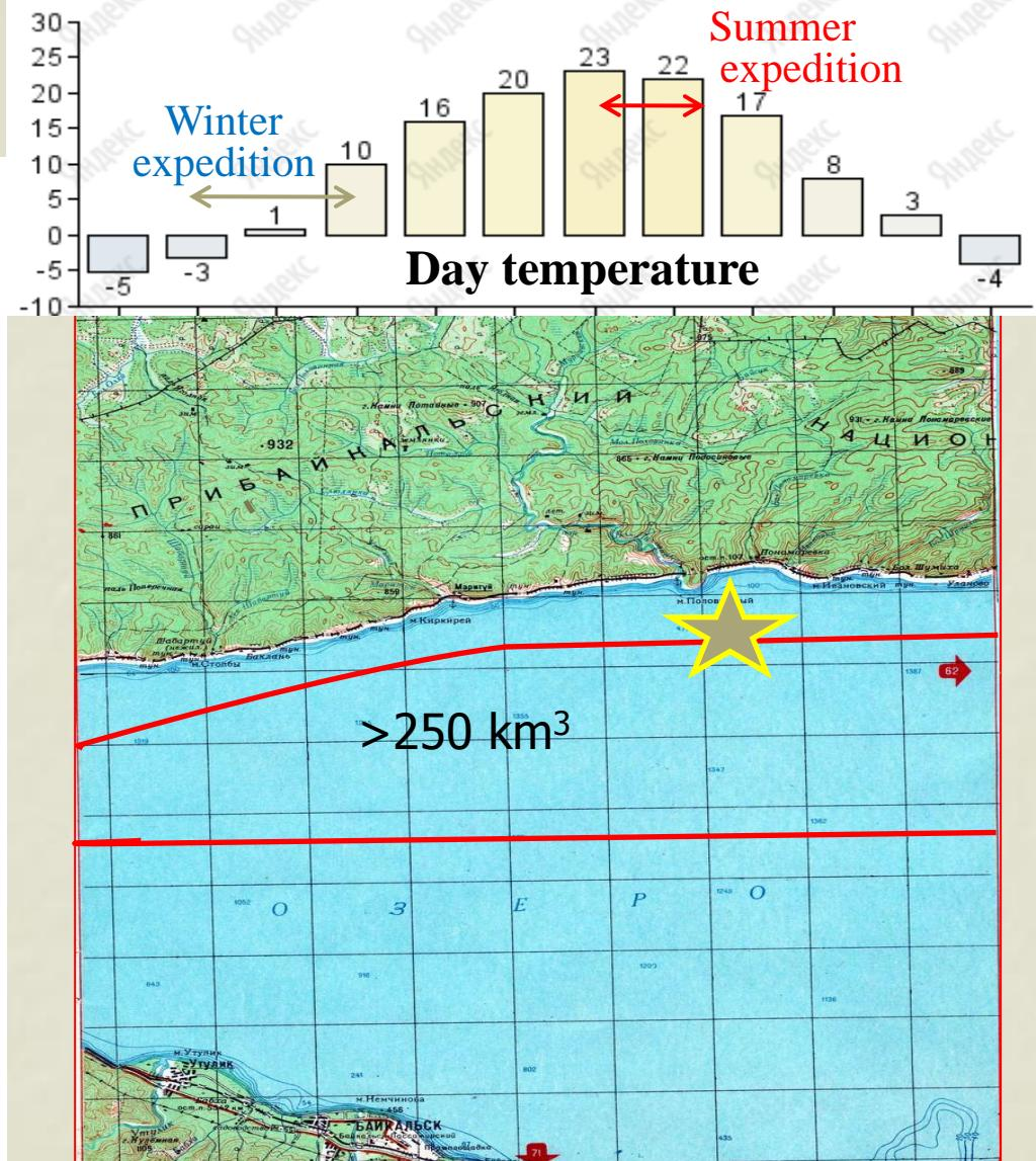
Depth – 1360 m; Flat the lake bed at  $>3 \text{ km}$  from the shore – allows  $>250 \text{ km}^3$  Instrumented Volume!
