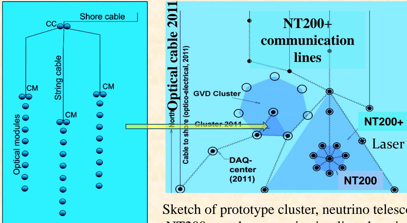
Sketch of prototype cluster, neutrino telescope NT200+, and communication lines locations.
