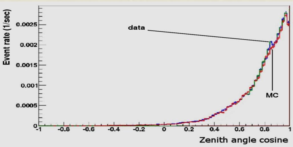
Zenith angular distributions of experimental and MC-simulated events after cut on  $\chi^2$  value
