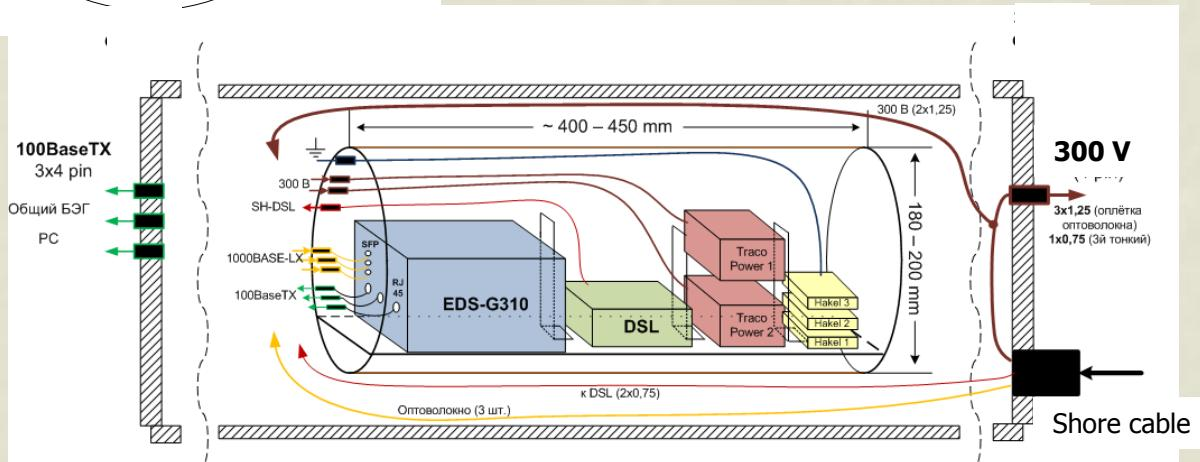
**Module of optical communication channel:** 2 data transmission channels 1 Gbit/c (3 optical fibers), 3 reserve optical lines, voltage supply (DC-DC TracoPower, MTBF  $3 \times 10^6$  hours).
