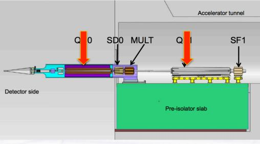
Natural ground motion: typical quadrupole jitter tolerance O(1nm) in main linac and O(0.1nm) in final doublet
