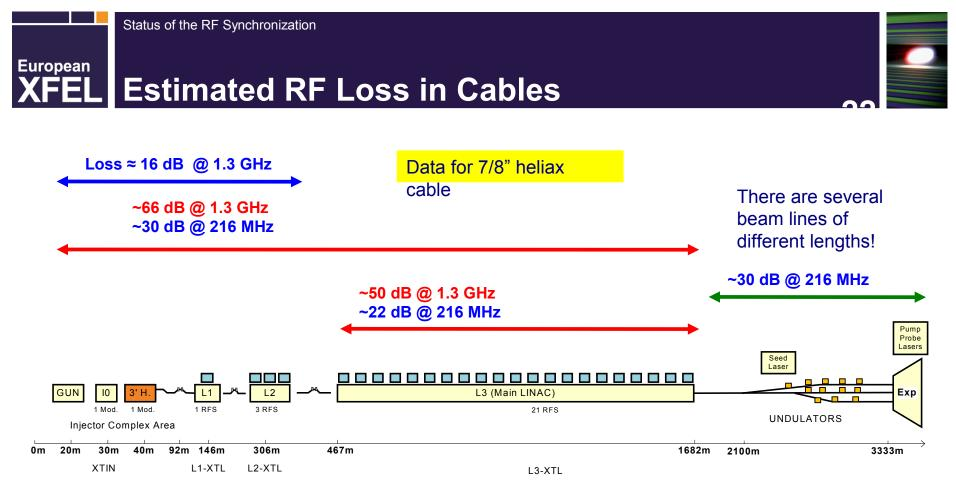
There will be 1300 MHz distribution up to L2 and 216 MHz after Main LINAC Two scenarios considered for Main LINAC:
