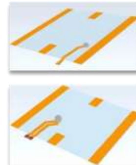
STEP 3: HV-tail Wire-bonding & Encapsulation
