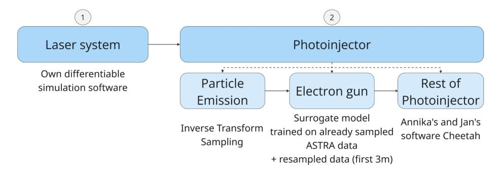
Possible way to model the whole system by interfacing the subsystems (1) and (2), derived from a discussion with Henrik.
