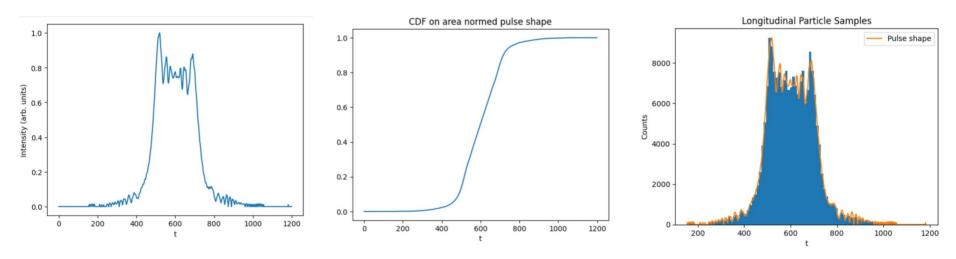
Inverse Transform Sampling from pulse shapes. From I.t.r.: laser intensity profile, cumulative distribution function of laser intensity profile, histogram of electron emission times sampled from intensity profile.
