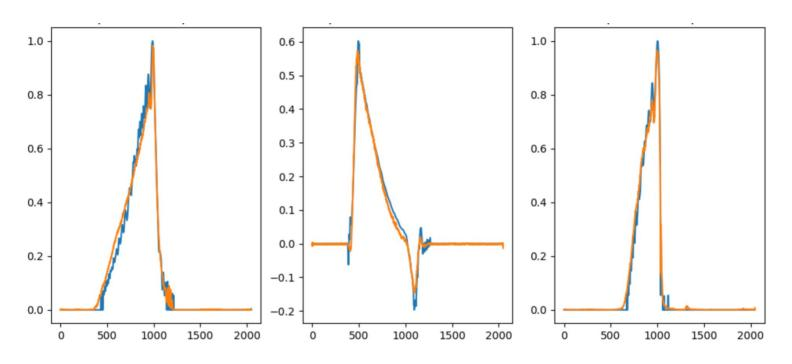
Multimodal VAE inference results, ground truth in blue, reconstructions in orange. From l.t.r.: Input pulse intensity profile, first derivative of the unwrapped input phase, output pulse intensity profile.
