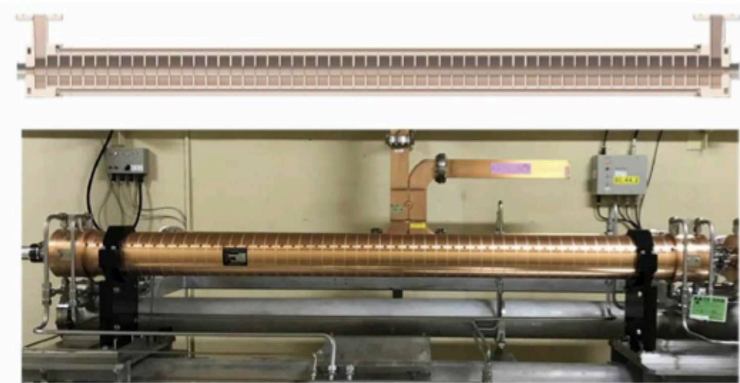
real S-band accelerating structure installed in a lab.
