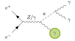
The energy of the **photon** from the  $\gamma/Z$  decay has a fixed value E, determined by the **recoil formula**
