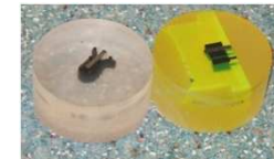
Cold mounted samples
