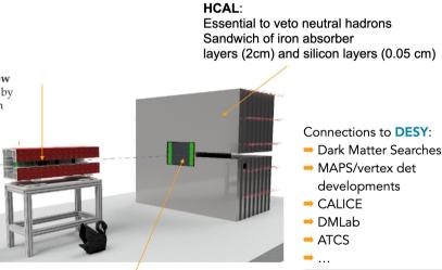
ECAL: SiW ECAL based on CALICE prototype
