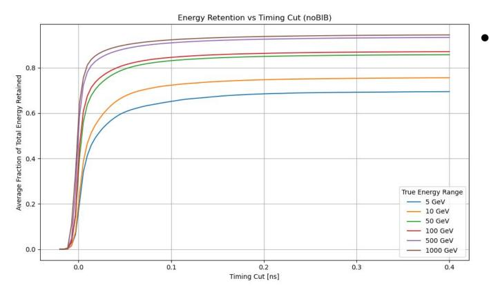
A timing cut of about 0.1 ns is needed to capture vast majority of the recoverable signal energy across the studied energy ranges
