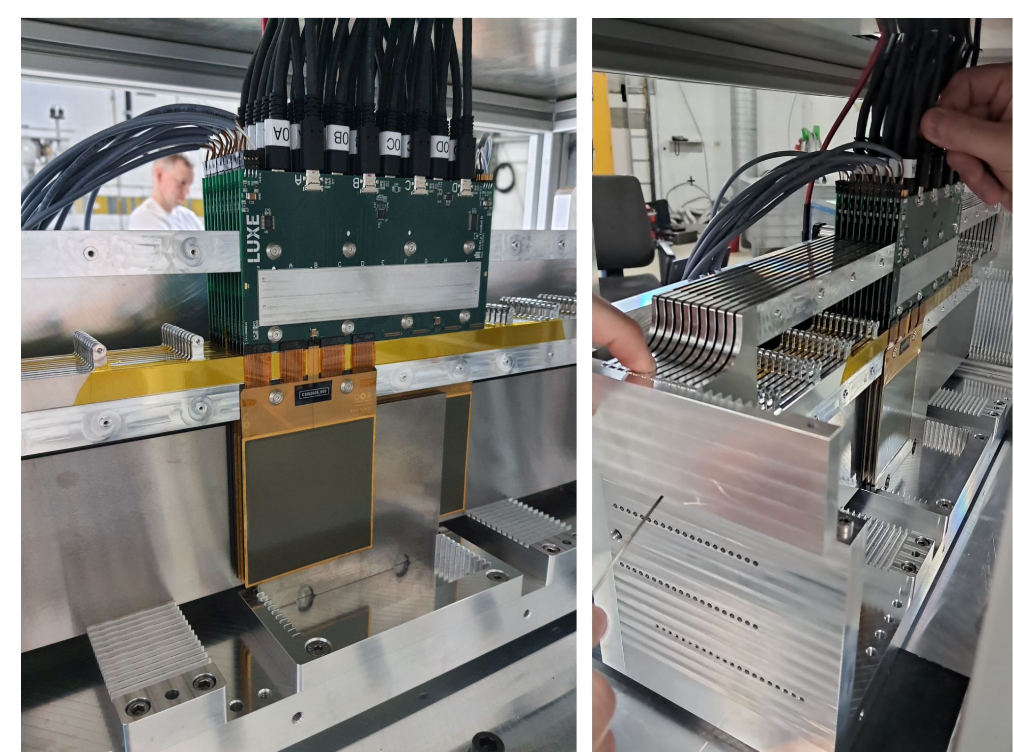
Fig. 8: ECAL-P prototype instrumented with two towers at DESY 5 GeV Test Beam in June 2025
