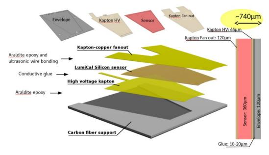
Figure 5.13. Structure of a sensitive layer of the LumiCAL calorimeter.
