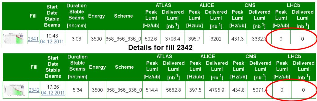
There are not collisions in LHCb, hence, the hits detected by sensor correspond to hits from beam halo and beam-gas interaction products.
