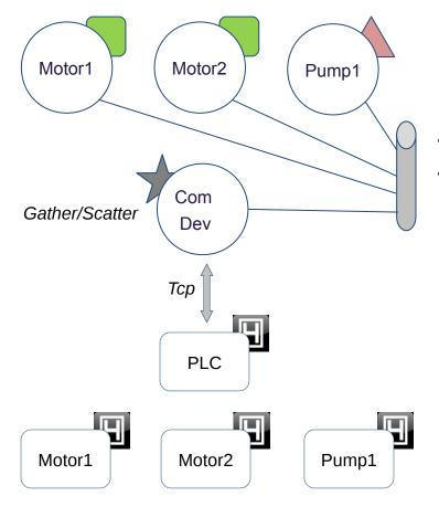
"Motor1", "signalPlcWrite" --- "ComDev", "slotPlcWrite" "ComDev", "signalPlcRead" --- "Motor1", "slotPlcRead"
