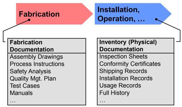
**Fabrication Documentation** for that **type of part**: Define how the part shall be realized (aka manufacturing dossier).
