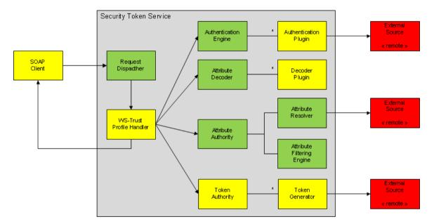
OpenSAML3 is used for producing and consuming the protocol messages The *green* components are / will be provided by Shibboleth 3 Identity Provider The *yellow* components are currently being implemented in the STS project
