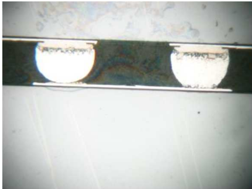
Too few UBM
