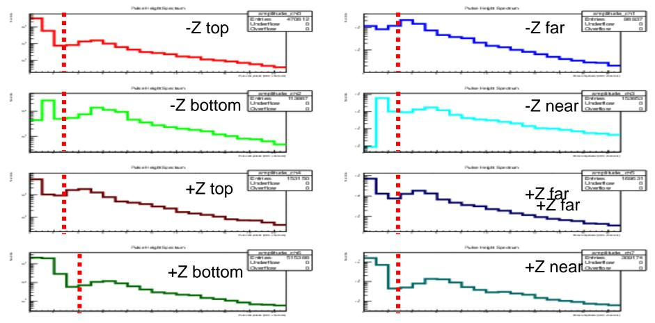
Thresholds in ADC spectra – threshold of 3 ADC counts shown. Corresponds to ~ 14 mV threshold of TDC.
