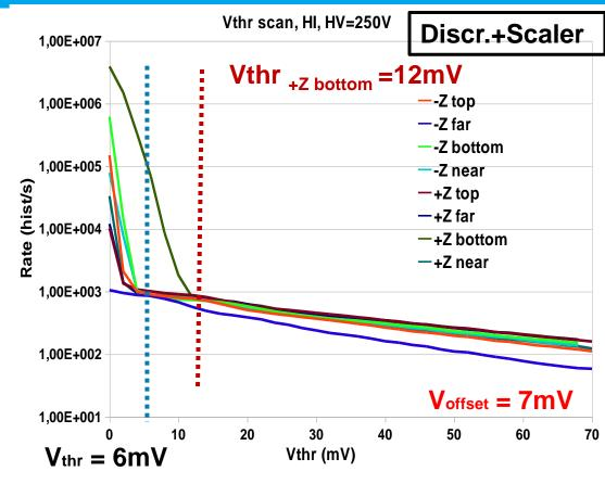
Measurements abore are without offset correction. Voffset ~7mV.
