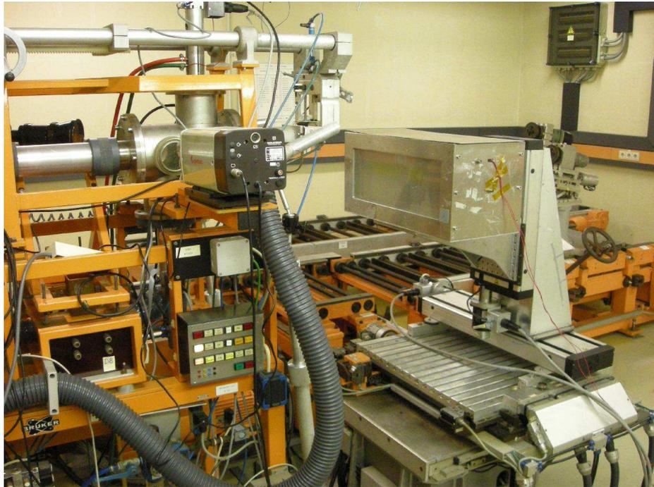
Irradiation box on XY-stage with beam line. Samples are fixed to Al-frames inside the box and scanned to reach uniform exposure.
