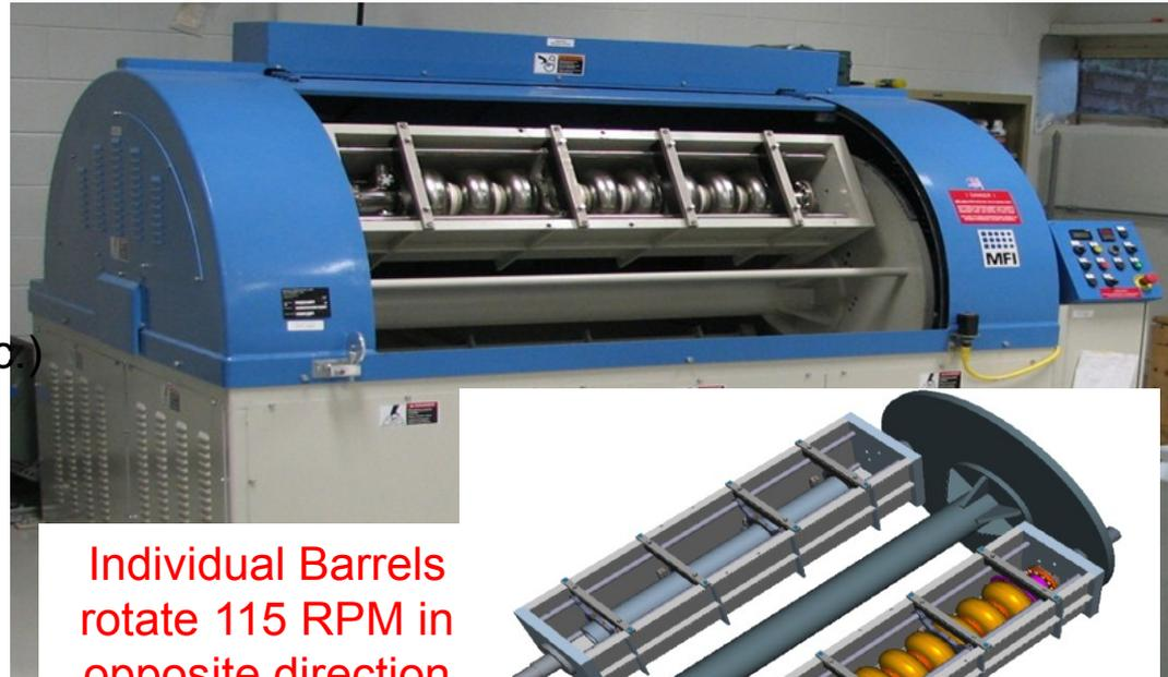
Individual Barrels rotate 115 RPM in opposite direction to main shaft
