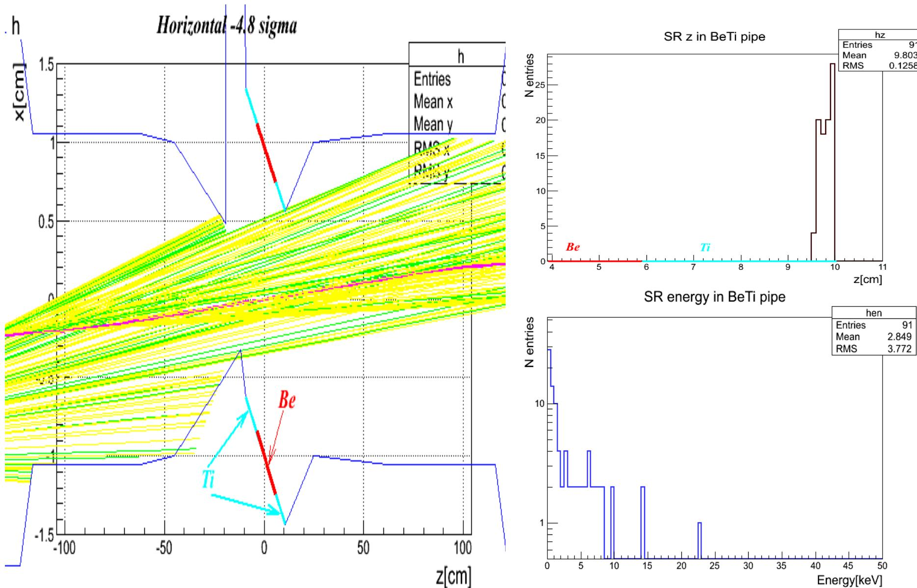
Orbit entering IP with  $\theta x/\sigma x = 0, +3, +6, +9, +12, +15, +18, \sigma x = 429 \mu\text{rad}$
