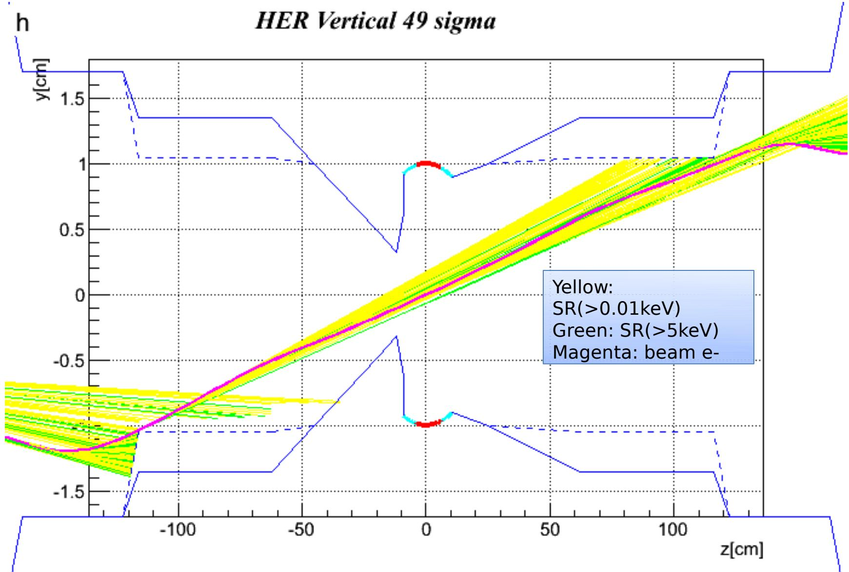
Orbit entering IP with  $\theta_y/\sigma_y = 0, +3, +6, +9, +12, +15, +18, +20, +25, +30, +35, +40, +45, +49, \sigma_y = 200\mu\text{rad}$
