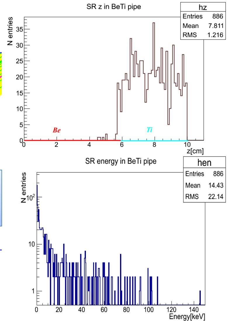
Assuming gaussian shape of beam angular distribution in X-plane, beam life time = 10min, and uniformly distributed halo electrons one can estimate number of direct hits of SR photons (>5keV) in Be -Ti beam pipe in case of gaussian beam core on top of uniformly distributed beam halo.
