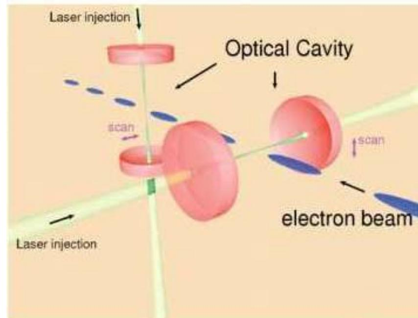
The advantage of the cavity based laser wire is laser wire stability ( position and wai
