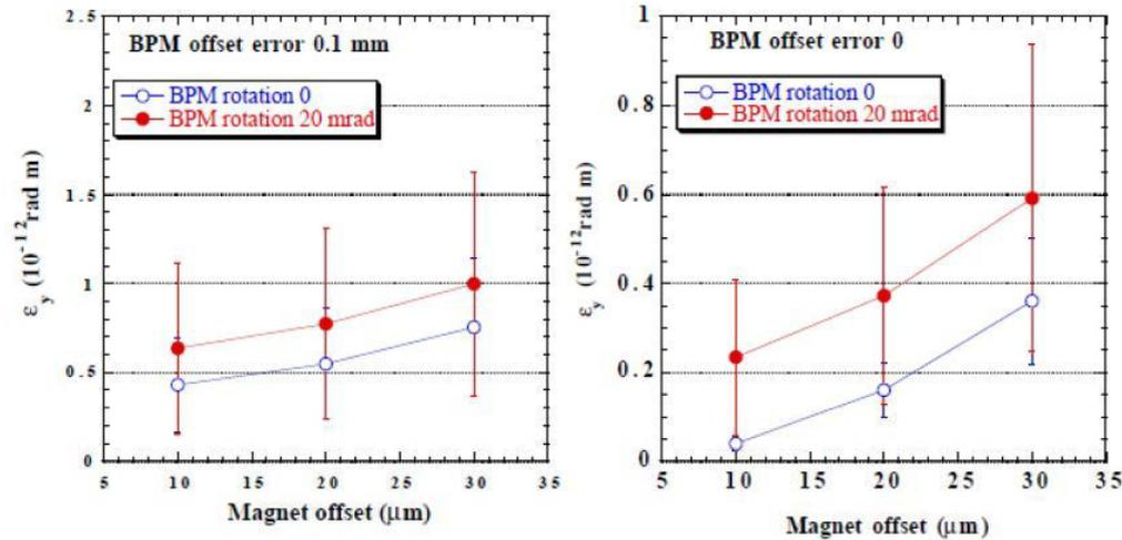
In order to achieve 1pm emittance, the magnet misalignment should be **less than 30um**.
