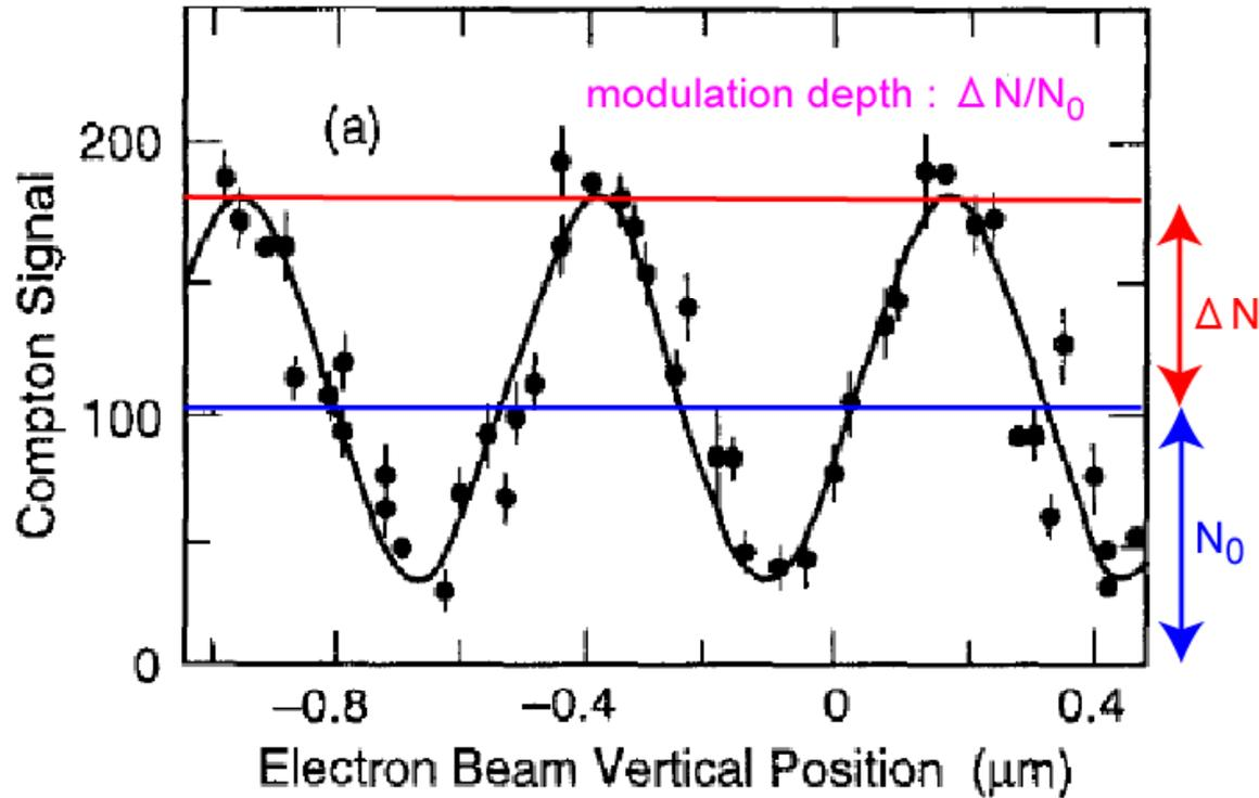
The 70nm beam size was measured in SLAC by laser interferometer.
