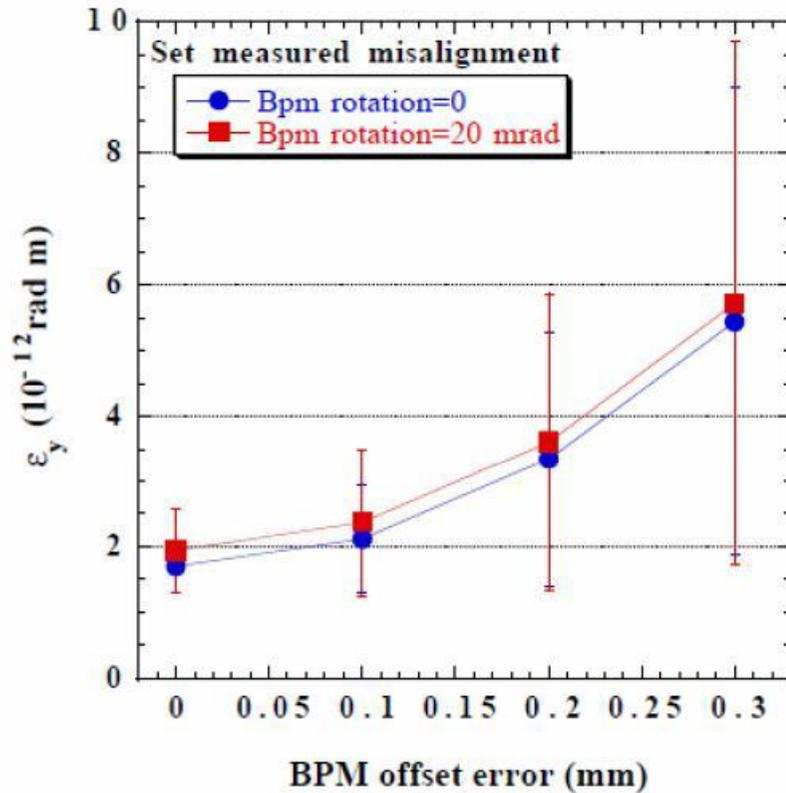
**BPM offset should be less than 100um.**
