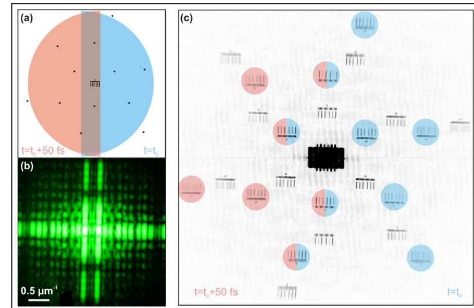
Two consecutive snapshots of an object, separated by 50 femtoseconds only, recorded in a single hologram exposure and disentangled afterwards
