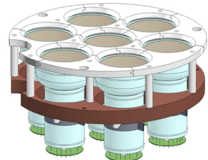
Prototype PMT mounting
