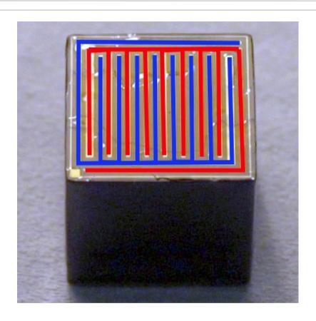
Two comb-shaped, differently biased anode grids create virtual "small pixel effect"
