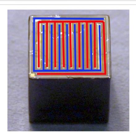
Two comb-shaped, differently biased anode grids create virtual "small pixel effect"
