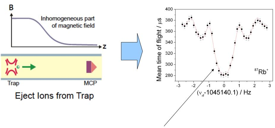
Minimum at cyclotron frequency
