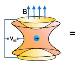
$\omega_c/2\pi$  = cyclotron frequency m = mass q = charge B = magnetic field strength
