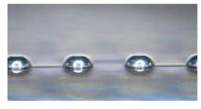
30 µm SnAg solder balls placed at PacTech.
