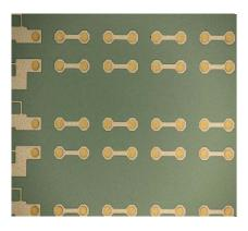
Our contact chain test structures made at CIS Erfurt with Ni-Au under-bump metal from PacTch
