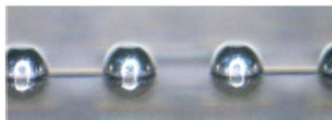
Side view of bumped daisy chain structure on chip
