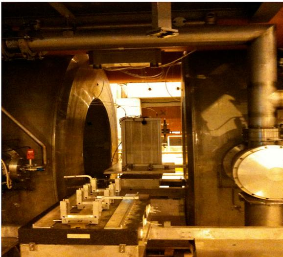
The Power-Pulsing mode was applied on a GRPC in a 3 Tesla field at H2-CERN (2ms every 10ms)
