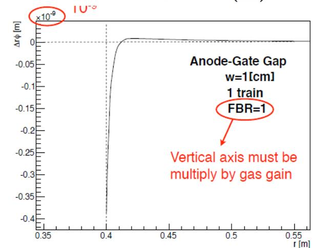
Distortions because of disk between MPGD – gating device are negligible.
