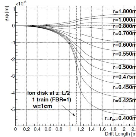
Ions from MPGD stage form 3 discs, if no gating devices is used  $\rightarrow \delta_{\max} \sim 60 \mu\text{m}$
