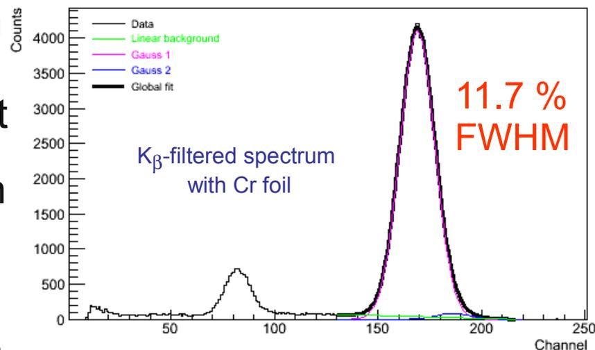
$^{55}\text{Fe}$  spectrum in Ar:CH<sub>4</sub> 90:10
