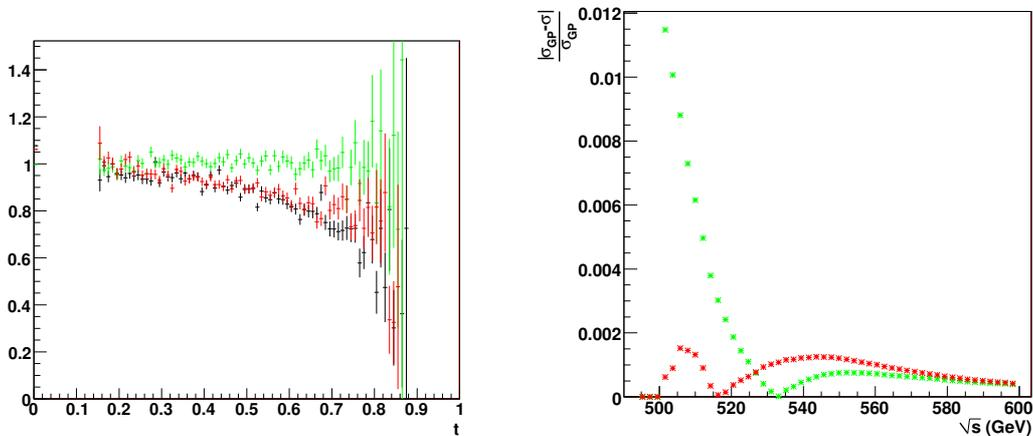
Figure 1: On the Left: The Ratios between the  $x_1$ -Distribution for  $x_2 = 1.0$  and the  $x_1$ -distribution for  $x_2 < 1.0$ . GP in Black, Circe in green, Correlated in Red. On the Right: The relative differences between GP and the circe parametrisation (green) and the correlated parametrisation (red) for a simple threshold scan. The Fit for the correlated parametrisation has been improved since the workshop.
