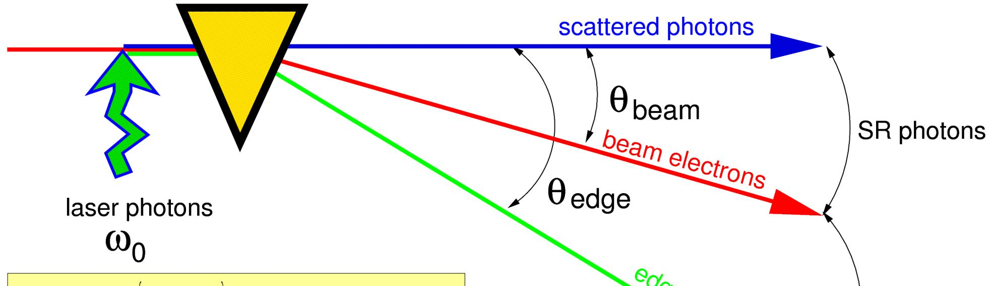
$$\left\{ \begin{array}{l} \theta_{beam} = \left( \frac{1}{E_{beam}} \right) \times \int B \cdot dl \\ \theta_{edge} = \left( \frac{1}{E_{beam}} + \frac{4\omega_0}{m^2} \right) \times \int B \cdot dl \end{array} \right.$$
