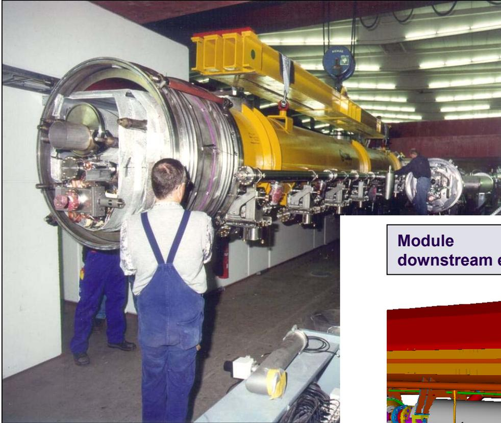
A real Accelerator Module at the “Tesla Test Facility” now called “FLASH”
