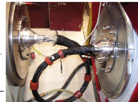
HV cable #2, leakage current ~ 50mA
