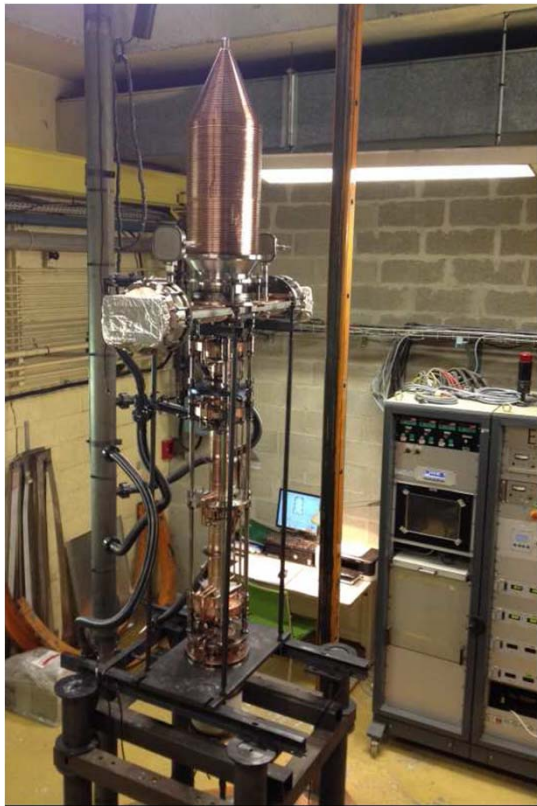
■ Klystron #1 before bake out
