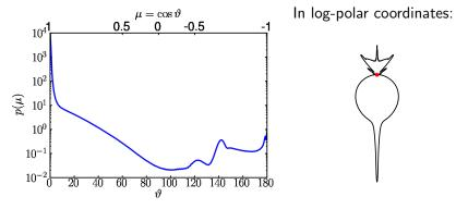
Example of water cloud phase function for  $r_{\rm eff}=10\mu$ m (wavelength  $\lambda\simeq 500$ nm)
