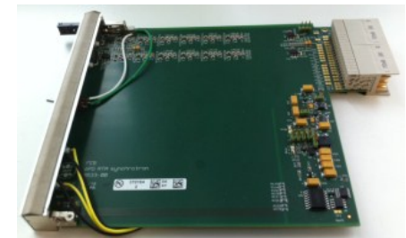
Pulse Stretcher RTM for SIS8300 (Peter Goettlicher, DESY)
