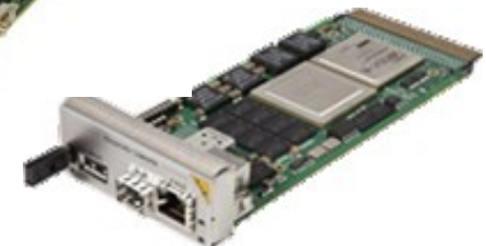
P4080 QorIQ based CPU with FPGA (N.A.T.)
