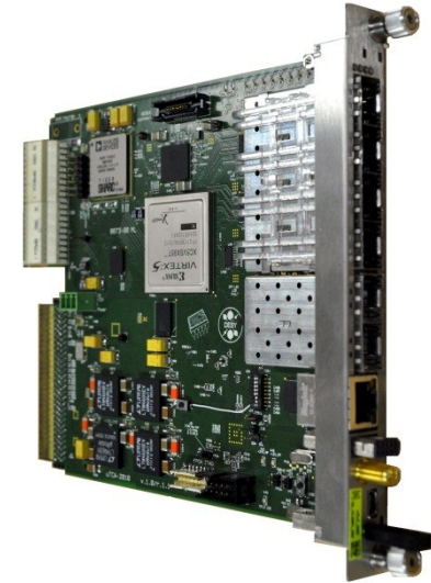
High-performance DSP and FPGA board (uTC) (DMCS/DESY)
