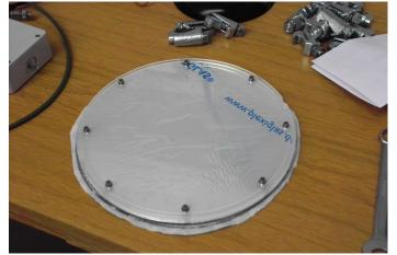
← Solar filter (10<sup>-5</sup>) fixed by two acrylic glass discs
