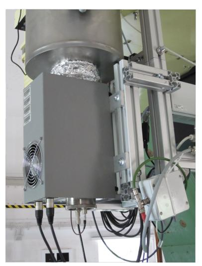
Flexible and easily adapted detector interface allows an uncomplicated variation of different detectors (CCDs and PMT cooler housing)
