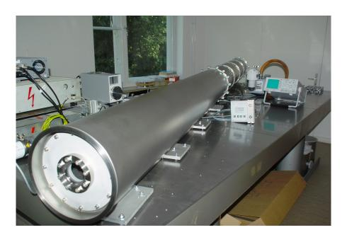
Vault structure tube assembled from 50 cm segments welded together.
