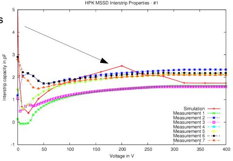
p-stop position is correct. Isolation thickness and concentration unknown. Other groups have not simulated p-stop capacities yet.
