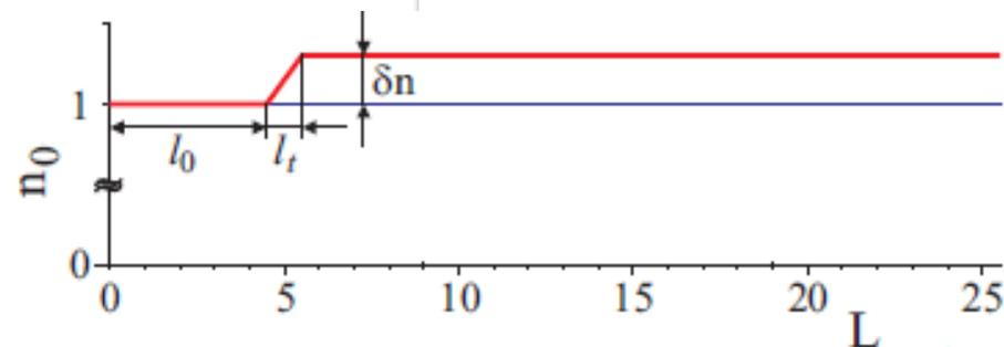
We will need precise control of plasma density ! Also needed for successful electron acceleration. Goal is 0.1-0.5% (still being defined).
