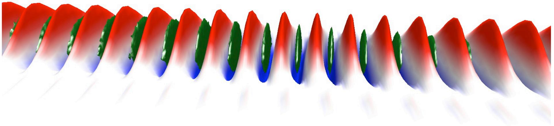
Side injection: high efficiency trapping of electrons, small energy spread
