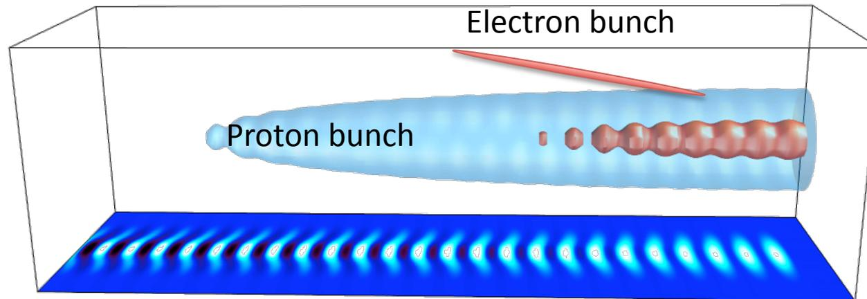
Electron bunch injected off-axis at an angle, so that it merges with the proton bunch once the modulation is developed and the phase velocity is high.
