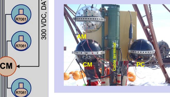
Commutation Module (CM): cluster trigger (4 FADC-200 MHz), strings power supply. Underwater PC: strings data transmission by DSLmodems. AM: communication
