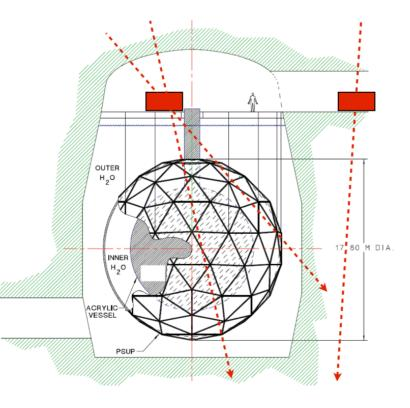
It is considered to install two different types of muon detectors above SNO+. One directly above the experiment to improve and externally calibrate the track reconstruction of through-going muons. Another station would measure muons passing close-by the detector through the rock. In coincidence with SNO+, a detection of muon-induced neutrons from rock would be possible. This would be the first measurement at this depth, with an average muon energy of  $\langle E_{\mu} \rangle \approx 350$  GeV.
