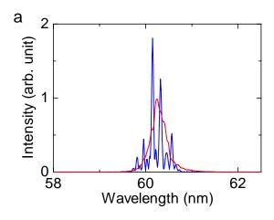
Spectrum measured at SCSS. Multi-longitudinal mode limits temporal coherency, which will be drastically improved by introducing seeding laser.
