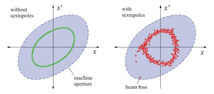
The dynamic aperture can be calculated from a tracking of the particles orbit through the accelerator where the nonlinear effect of sextupole magnets has to be treated as step by step correction in linear beam matrix optics:
