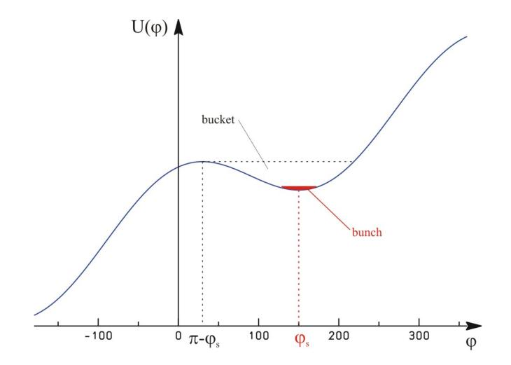
$\varphi_1^{\max} = \pi - \varphi_0$  is an extreme elongation corresponding to a stable motion. The corresponding curve in phase space is called separatrix and the area delimited by this curve is called the RF bucket. Part of this area is filled with particles, forming the bunch.
