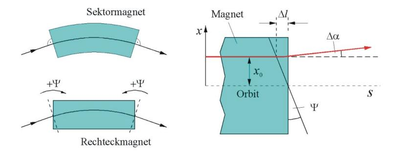
For a deflection angle  $\varphi$  we have an entrance and exit angle  $\psi = \varphi/2$ . The orbit of a particle traveling with a radial displacement  $x_0$  at the position of the magnet pole of a rectangular dipole is shorter than the reference orbit (with  $x_0 = 0$ ) by
