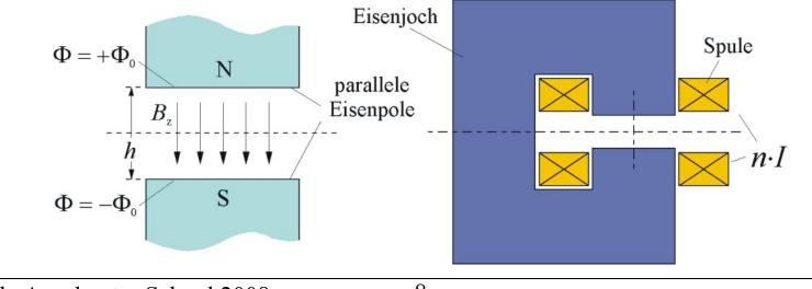
Typical types of dipole magnets are the C-Magnet, the H-Magnet and the Window-Frame Magnet:
