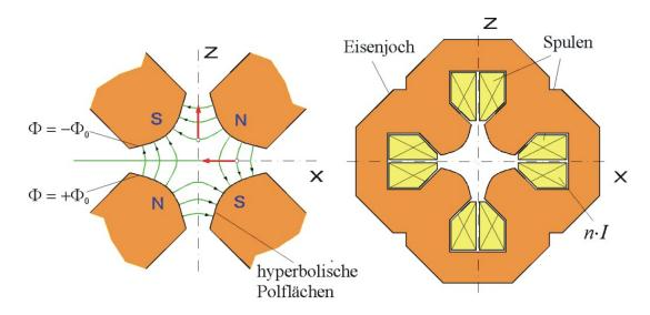
The magnetic field inside the gap is determined from the gradient of the magnetic
