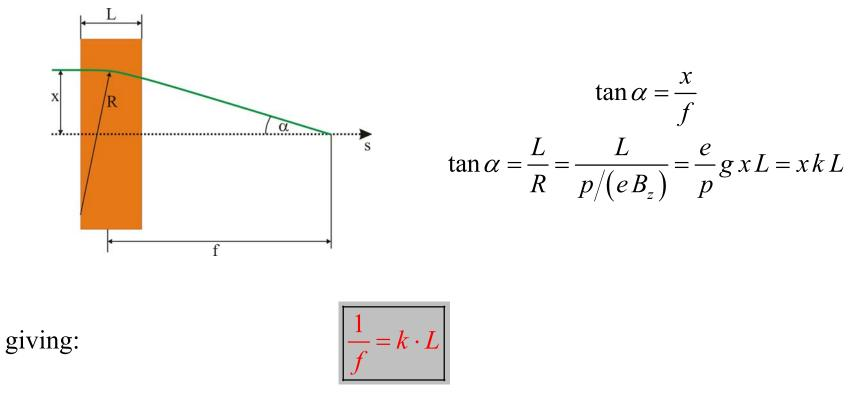
Here we have assumed the length L to be short compared to the focal length f such that R does not change significantly within the quadrupole magnetic field.
