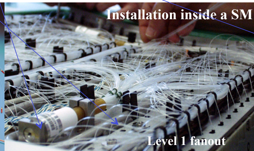
Optical fiber harness : 200 fibers => 200 crystals
