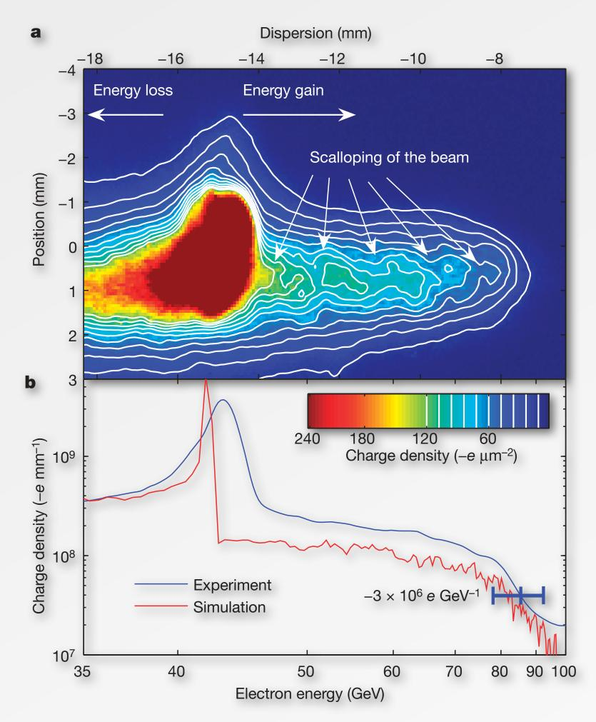
Energy doubling of 42 GeV electrons in a metre-scale plasma wakefield accelerator
