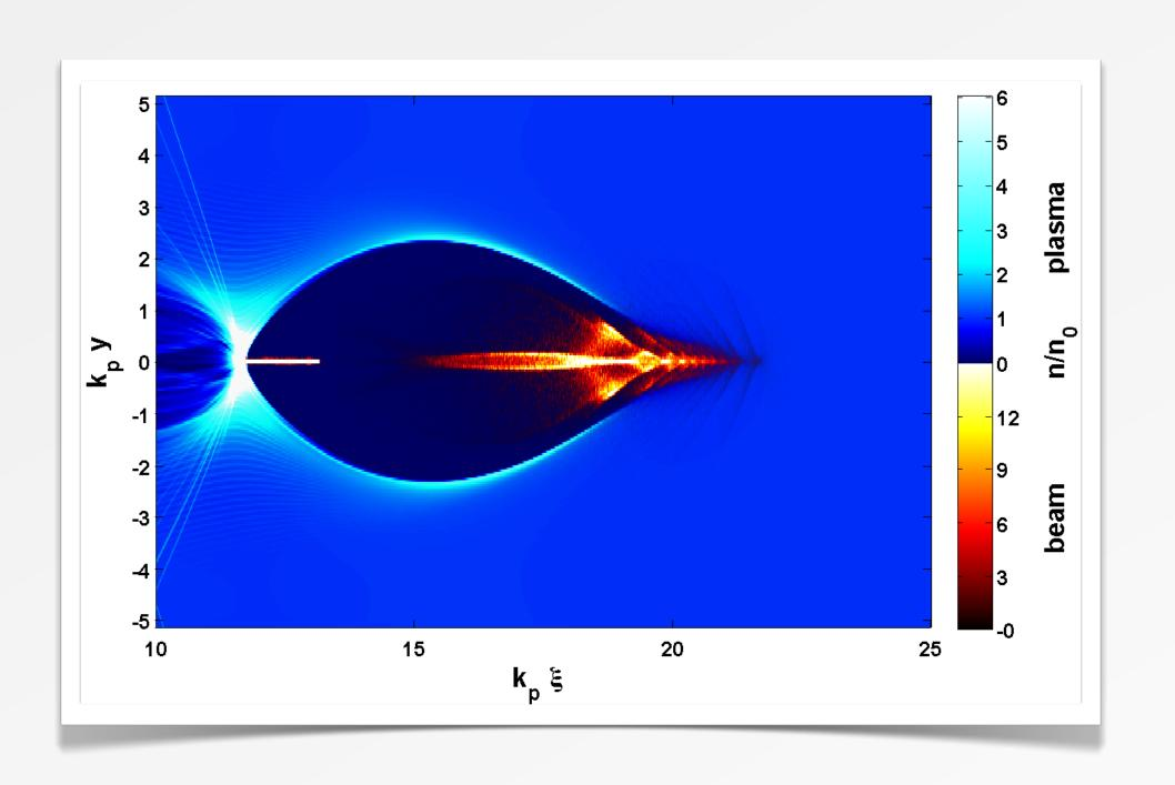
HiPACE simulation with dynamical time-step adjustment
