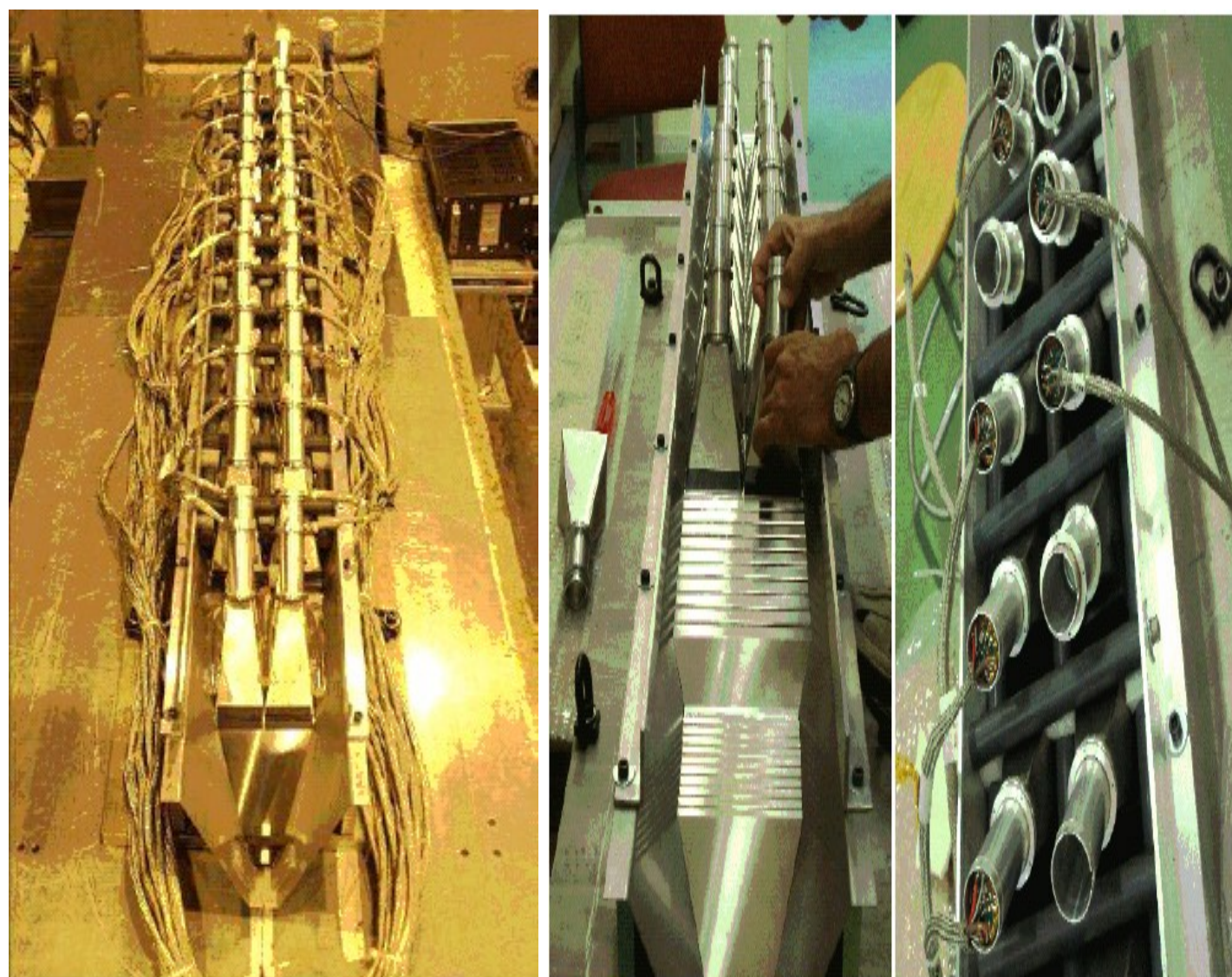
Figure 1. Photograph of the fully instrumented octant prototype at the beam test (left) and successive stages of the octant calorimeter assembly with W/Q-plates, air-core light guides and PMTs (left & right)
