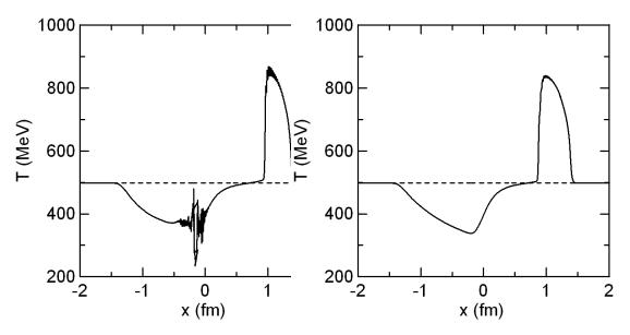
Fig. 1: The temperature in the shock formation calculated without the finite size effect (left) and with the finite size effect (right), starting from the homogeneous initial condition (dotted line) [6].
