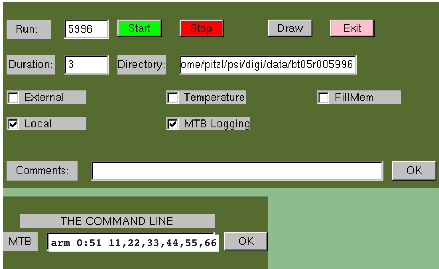
**activate test pulse for columns 0..51 in 6 rows**
