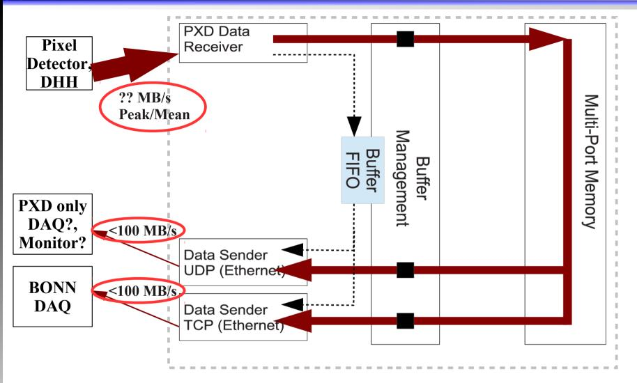
Data in format: DHP/raw, zero/not-zero suppressed
