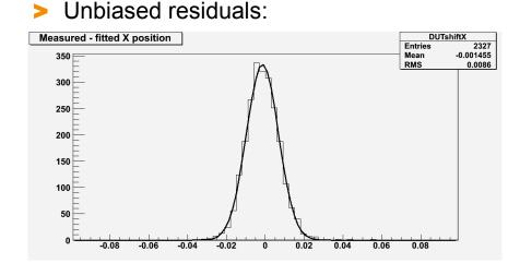
d = 150mm,  $\sigma \sim 8 \mu m$
