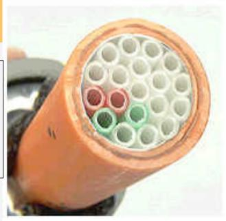
Sheath tube with internal capillaries
